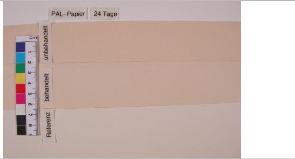
Figure 3: Aging properties of the PAL paper (image taken from paper treated in batch 1). Treatments are as follows: “Unbehandelt”: untreated, aged* “Behandelt”: treated with Booksaver®, aged* “Referenz”: untreated and unaged * 24 days at 80°C and 65%RH (DIN/ISO 5630:3)
